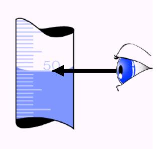
Second, read the volume at the bottom of the meniscus, (the curve in the surface of the liquid) if the curve is downward.
