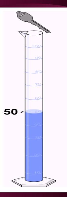
Step 3: Take a new volume reading. The difference in the two volume readings is the volume of the key. (53 ml - 50 ml = 3 ml)
